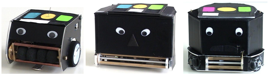
Fig. 1. Different robots designs. From left to right: classical two wheeled design, two wheeled defender, and robot with omnidirectional drive.
