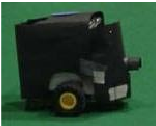
Fig. 1. An image of one of the robots of the 4 STOOGES. The Eyebot controller is mounted on the top.
