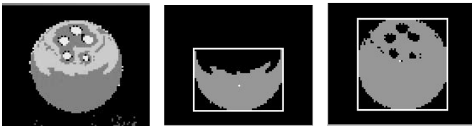
Fig. 2. Left: Ball with original, white and mixed colour ( yellow-orange ) regions. Middle: Bounding box extracted with last year vision system. Right: Ball original colour region after merging related connected components, and resulting bounding box extracted.
